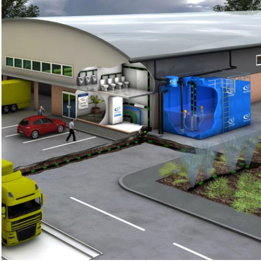
Fig 2. Above ground rainwater harvesting system
